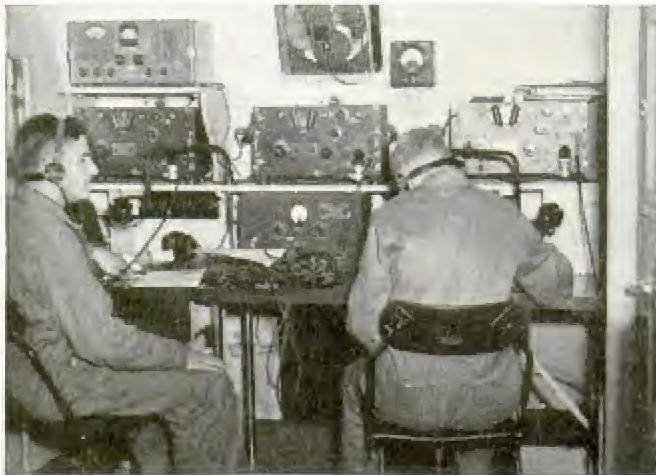
Above, interior view of the "broadcasting station on wheels" (below) used by the Signal Corps. Trailer carries radio receiver, also motors to supply power for a transmitter in the tractor
